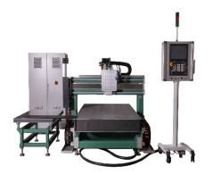
The glass processing systems of the LD series from MDI Advanced Processing GmbH offer high-quality processing of brittle materials for a variety of industrial applications due to the laser technology used (532nm).
